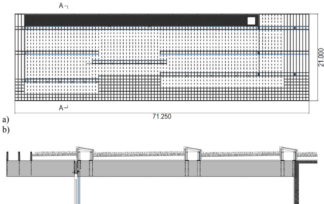
Figure 2: a) plan view and b) view of a transverse beam with a span of 13.50 m and a cantilever of 4.50 m (cross section A-A in plan view)
