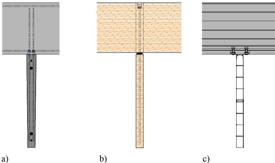
Figure 3: Cross-section of the transverse beams and view of the longitudinal stiffeners for the three investigated options: (a) ultra-high performance fibre reinforced concrete, (b) timber beams and (c) extruded aluminium profiles
