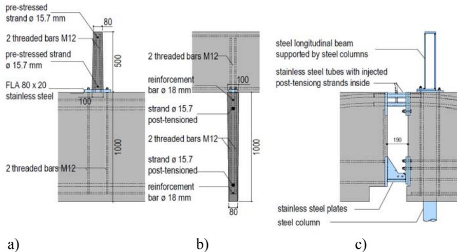
Figure 5: a) and b) detail of joint between longitudinal and lower transversal beams and c) detail of thermic joint and of the suspension of transverse beams to the steel beams
