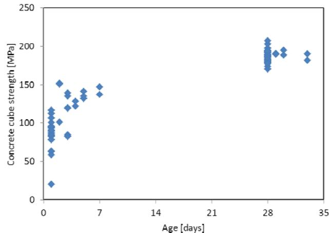
Figure 6 : Compressive strength measured on 100x100x100 mm cubes as a function of the concrete age
